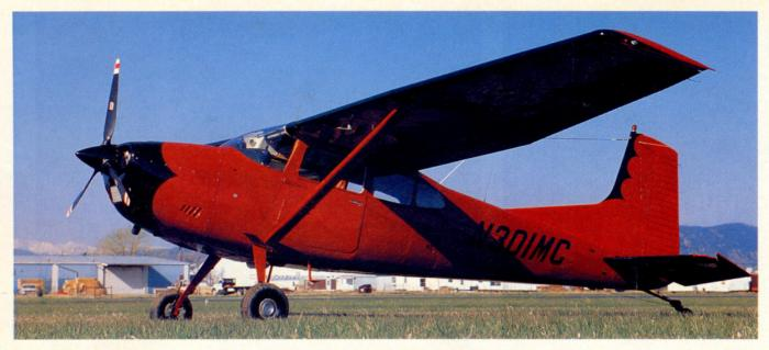
duction, Cessna offered Continental's 300-hp (285 hp continuous) IO-520 as an option and, not surprisingly, the deeper-voiced 185 quickly eliminated its weaker sibling on the Pawnee assembly line in Wichita.
